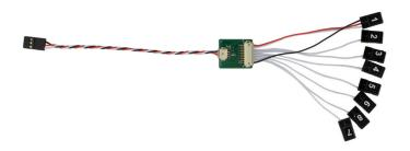
Connect the three-wire cable to your autopilot's input pins.
