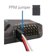
signal (s) white wire power (+) red wire ground (-) black wire When powered, the LED indicates the status of the radio signal.
