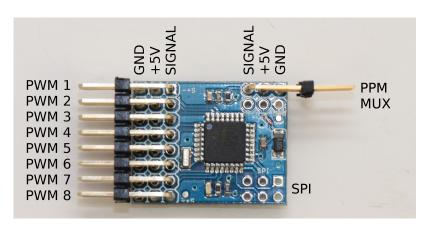
Connect the PWM signals coming from your receiver to the inputs. The "S+-" next to the pins indicates the polarity.
