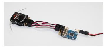
Or use a <u>2 pin jumper cable</u> for +5V and ground, and a <u>5</u> or <u>6 pin jumper cable</u> for the signals:
