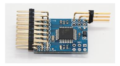
Use a 3x8 right angle pin header for the PWM connections and a 3x1 right angle pin header for the PPM connection (or a 3x2 right angle pin if mux connection is needed).
